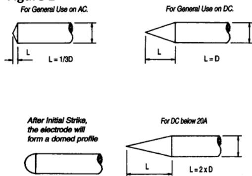
Further advice on recommended electrode types, tip configuration and process variations are available in the Parweld TIG / GTAW process synopsis on [www.parweld.com](http://www.parweld.com).
